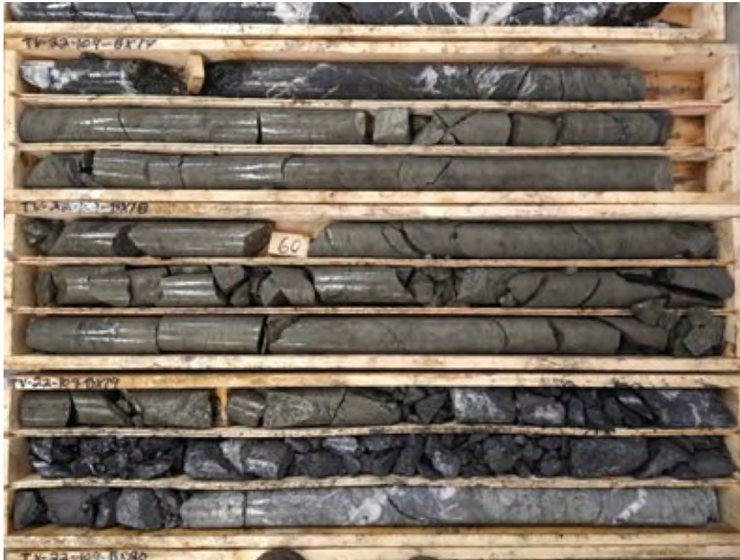
Figure 5. TV22-109 ~55-65 m showing a mudstone-hosted massive sulfide intercept. Sulfide mineralization begins ~10 m above the massive sulfide horizon, and is characterized by ~20% pyrite hosted within sheared peperitic andesite and dacite. The massive sulfide is underlain by faulted mudstone and andesite breccia, both of which contain appreciable stockwork-style sulfide mineralization. Handheld XRF analyses of the massive sulfide show very high concentrations of the Au pathfinder elements Ag, As, and Sb. Handheld XRF cannot reliably measure Au concentrations.
