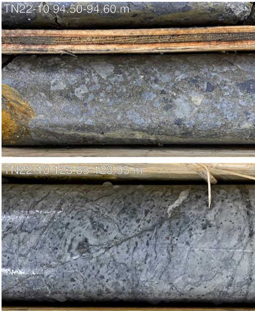
Figure 10. TN22-10 94.50-94.60 showing a close-up of semi-massive replacement-style mineralization hosted by rhyolite breccia. This type of sulfide mineralization shows the highest pathfinder element concentrations. TN22-10 123.85-123.95 showing stockwork sulfide and vesicle-hosted disseminated sulfide mineralization. This style of mineralization is ubiquitous at Tarn Lake. Accurate handheld XRF analyses of disseminated mineralization is impossible given the small size of the disseminations and consequent mixed analyses of sulfide and host silicate material. Analyses of larger stockwork veins throughout the Tarn Lake drill holes shows the presence of Ag, suggesting that disseminated sulfides may host Ag as well.
