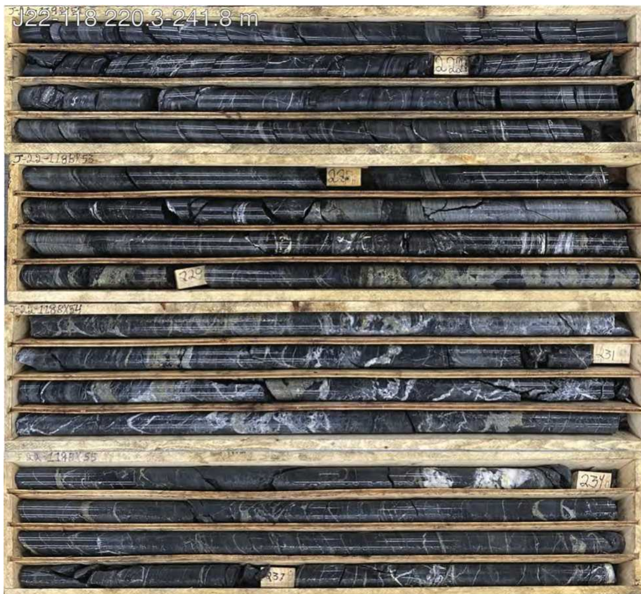
Figure 3. J22-118 220.3-241.8 m showing stockwork sulfide mineralization with hydrothermal silica, hosted by an intensely silicified mudstone. This intercept is polymetallic, with abundant chalcopyrite and sphalerite filling fractures within pyrite. Investigations with handheld XRF show consistently high values of the pathfinder element Ag, particularly in chalcopyrite-rich zones. Gold concentrations cannot be reliably measured with handheld XRF.
