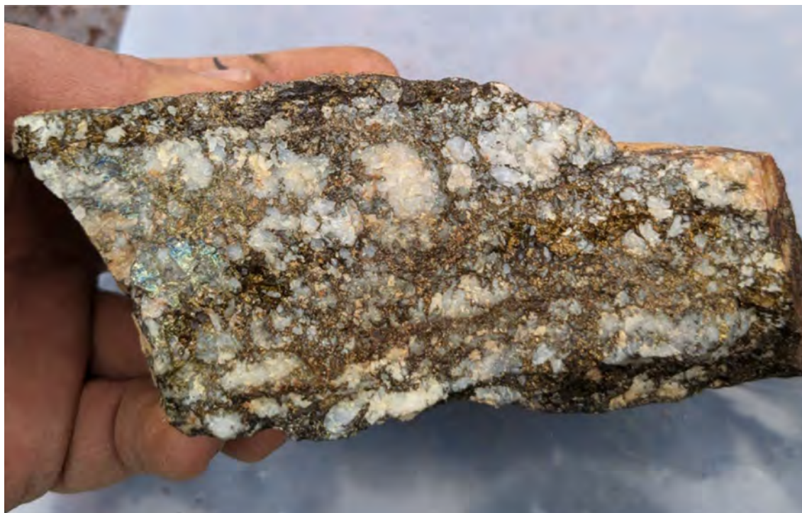
Figure 3 – A piece of quartz-carbonate-sulfide vein material from a select sample collected at Vermillion. This sample grades 205 gpt Au and 0.7% Cu. The vein was traced along surface for approximately 200m.
