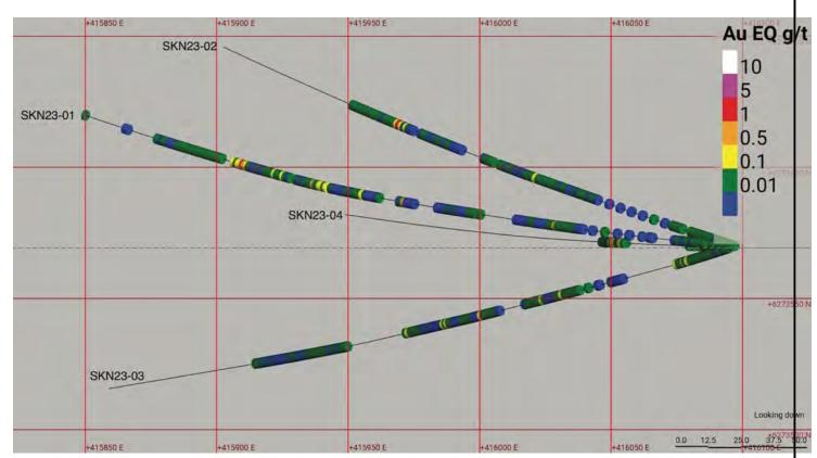
**Figure 11:** A plan-view map showing down-hole assay results in Au equivalent for 2023 drilling at Scarlet Knob. Mineralized intercepts near the bottom of SKN23-01 and SKN23-02 are associated with a contact between silicified Eskay rhyolite and unaltered mudstone, suggesting the presence of a paleoseafloor contact at this location.
