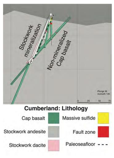
**Figure 4:** A cross-sectional view looking along strike showing the lithologies intercepted by drilling in 2023. The black dashed line indicates the mineralized paleoseafloor contact between the stockwork andesite and the non-mineralized, highly magnetic pillow basalt that caps VMS mineralization.
