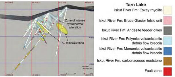
**Figure 9:** A cross-sectional view of Tarn Lake looking south showing lithologies intercepted by drilling in 2022-2023. Intense hydrothermal alteration and Au mineralization is associated with Eskay rhyolite cut by east-west trending andesite dikes. Sedimentary rocks intercepted are generally weakly- to non-altered and non-mineralized.
