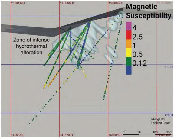
**Figure 10:** A cross-sectional view of Tarn Lake looking south showing measured magnetic susceptibility values in drill holes from the 2022-2023 program. There is a strong correlation between zones of intense hydrothermal alteration, Au mineralization, and weak magnetic susceptibility. These observations are consistent with hydrothermal destruction of magnetic minerals in a VMS feeder zone.
