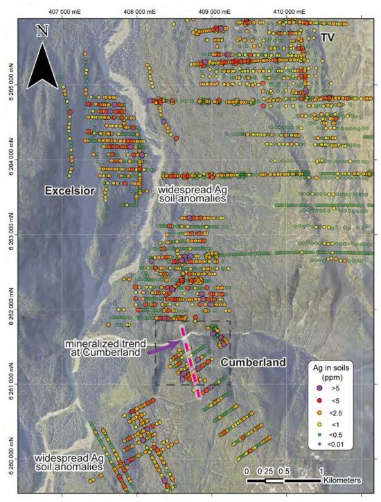
**Figure 5:** Map showing soil sampling conducted in the Cumberland, Excelsior, and TV regions during the late 1980's and early 1990's, as well as recent soil samples collected during the 2021-2022 exploration programs. The mineralized trend identified by drilling at Cumberland extends towards areas with Ag anomalism, suggesting mineralization at Cumberland may extend along strike, particularly to the southwest.
