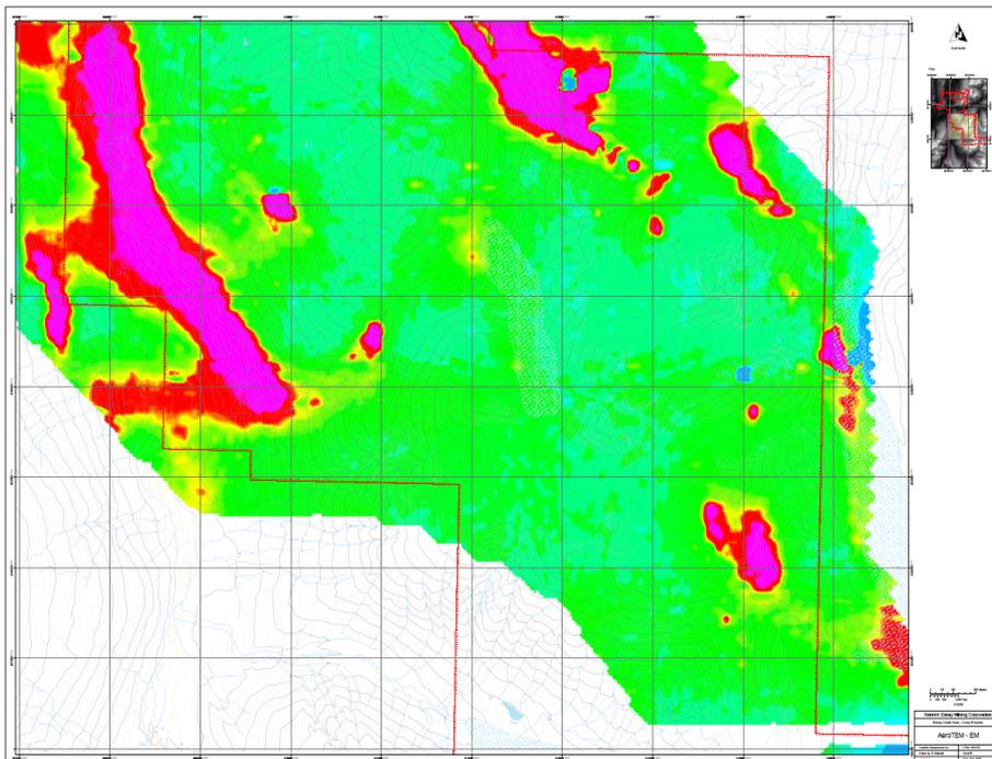
**Figure 13.** AeroTEM© II EM data for the Corey Property survey area, split into contiguous north and south sheets (red line indicates property boundary).
