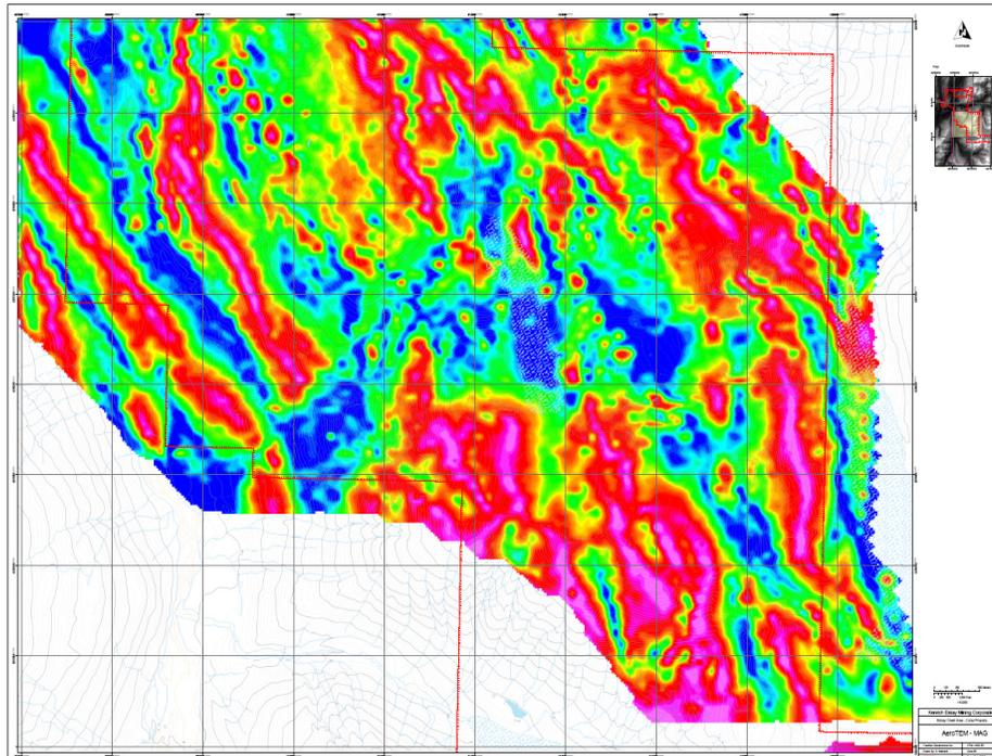
**Figure 14.** AeroTEM<sup>®</sup> II TMI data for the Corey Property survey area, split into contiguous north and south sheets (red line indicates property boundary).
