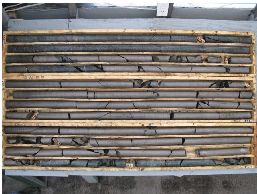
**Photo plate 4: Detail of the network vein style mineralization in the 65.5-69.7 metre interval of drillhole RL-3**
