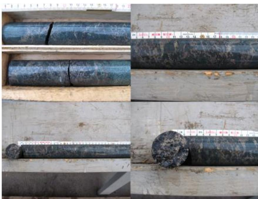
**Photo plate 5: CR08-88, part of the ~239.6-244.4 metre interval; "Eskay Style" hydrothermal brecciation**
