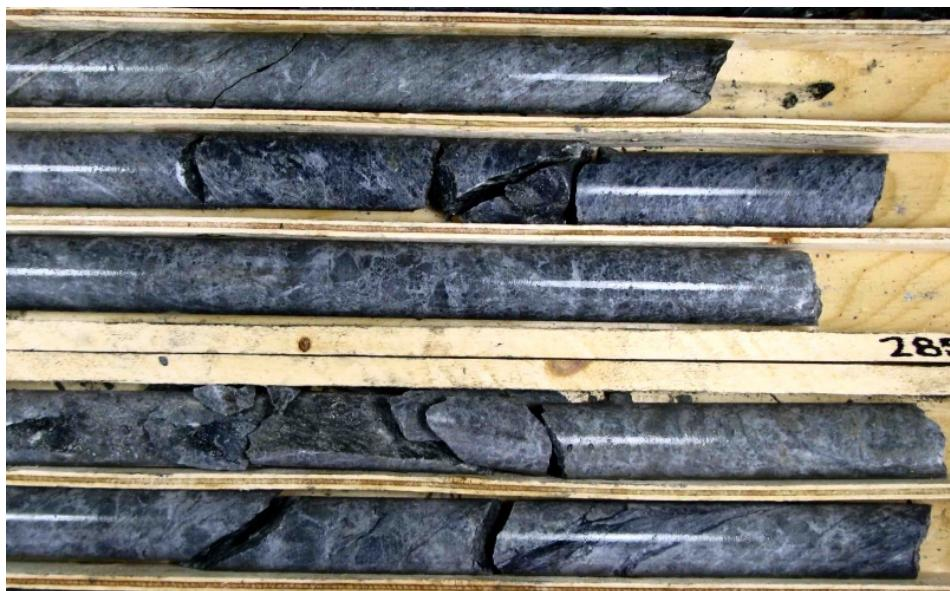
**Photo plate 6: CR08-86, part of the ~281.2-291.0 metre interval; "Eskay Style" hydrothermal brecciation**
