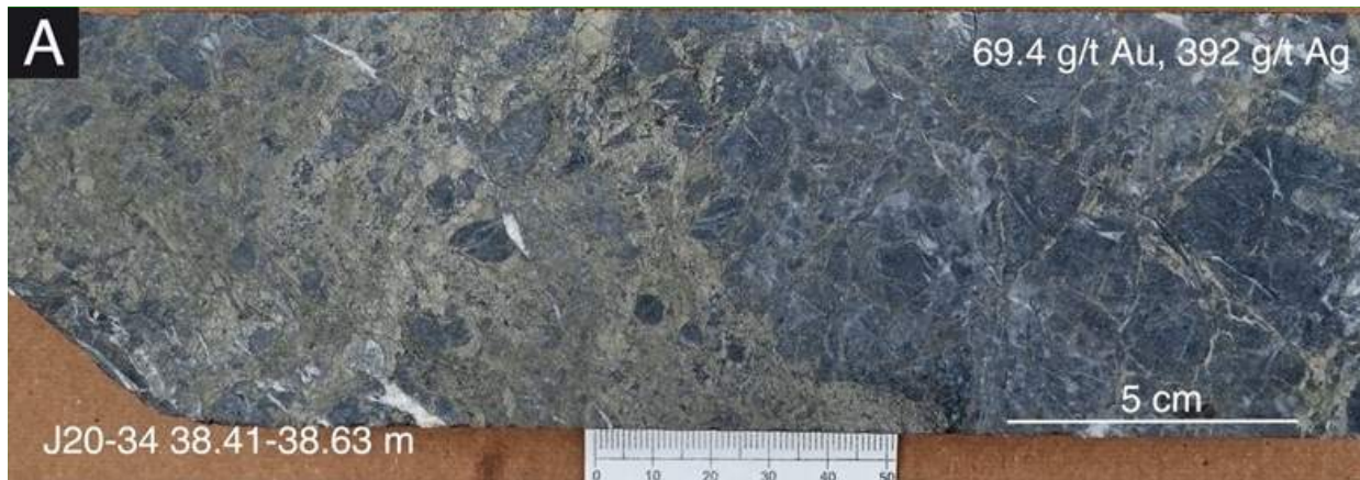
High Au-grade cut and polished core, from 2020 Drilling at the Jeff Zone
