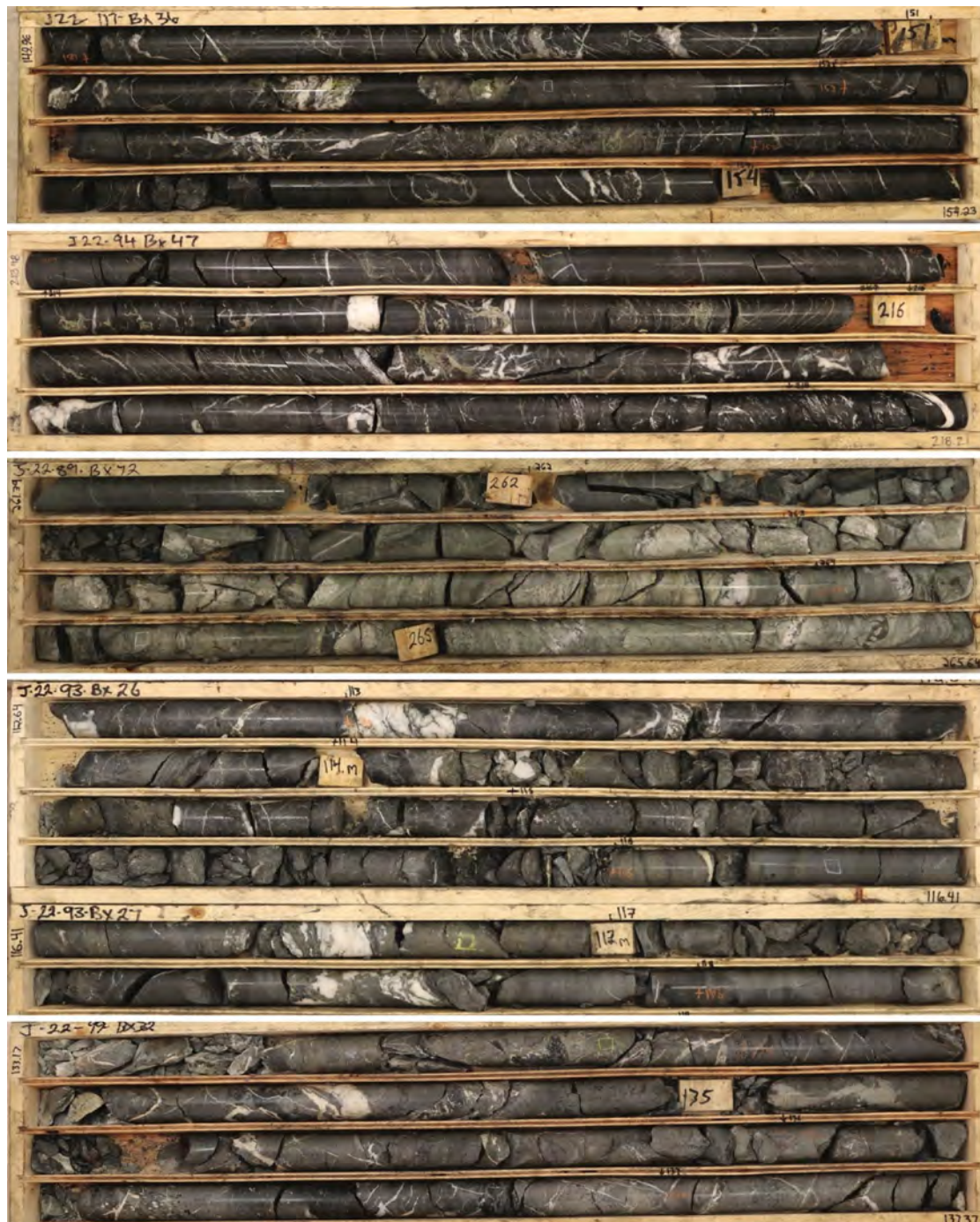
Figure 3. Representative examples of stockwork-style mineralization intercepted at Jeff North. These drill holes intercepted a 750 m long corridor of VMS mineralization and intense hydrothermal alteration at stratigraphically equivalent horizons to those at TV and Jeff.
