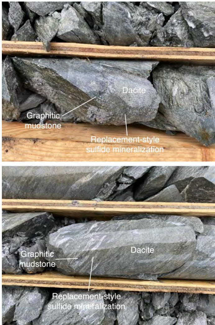
Figure 13. Sulfide mineralization hosted by intensely sheared peperitic dacite. Sulfide minerals have been recrystallized and formed banded aggregates of ~1mm pyrite crystals.
