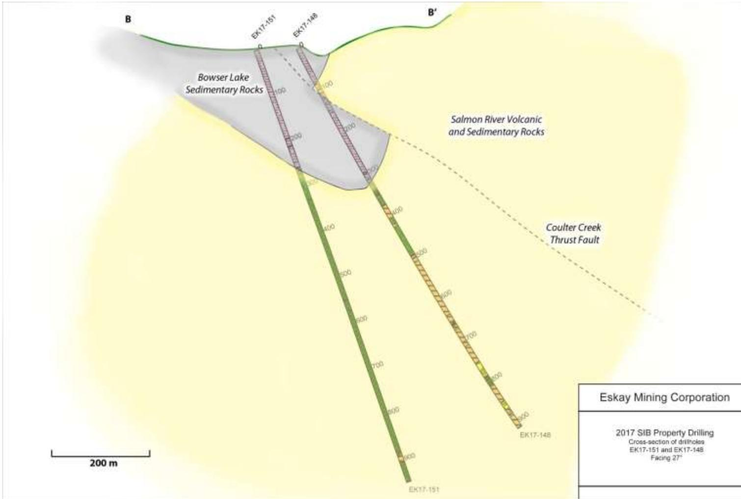
Figure 3: Vertical cross-section of holes EK17-151 and EK17-148, striking 117 degrees
