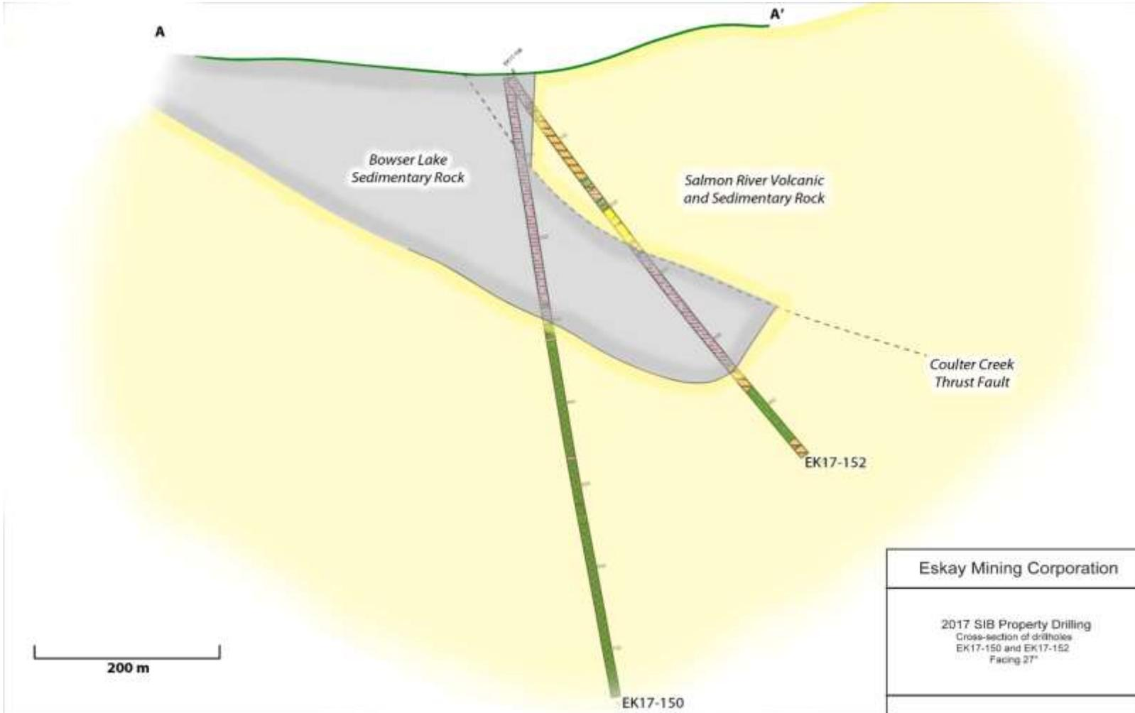
Figure 2: Vertical cross-section of holes EK17-150 and EK17-152, striking 117 degrees
