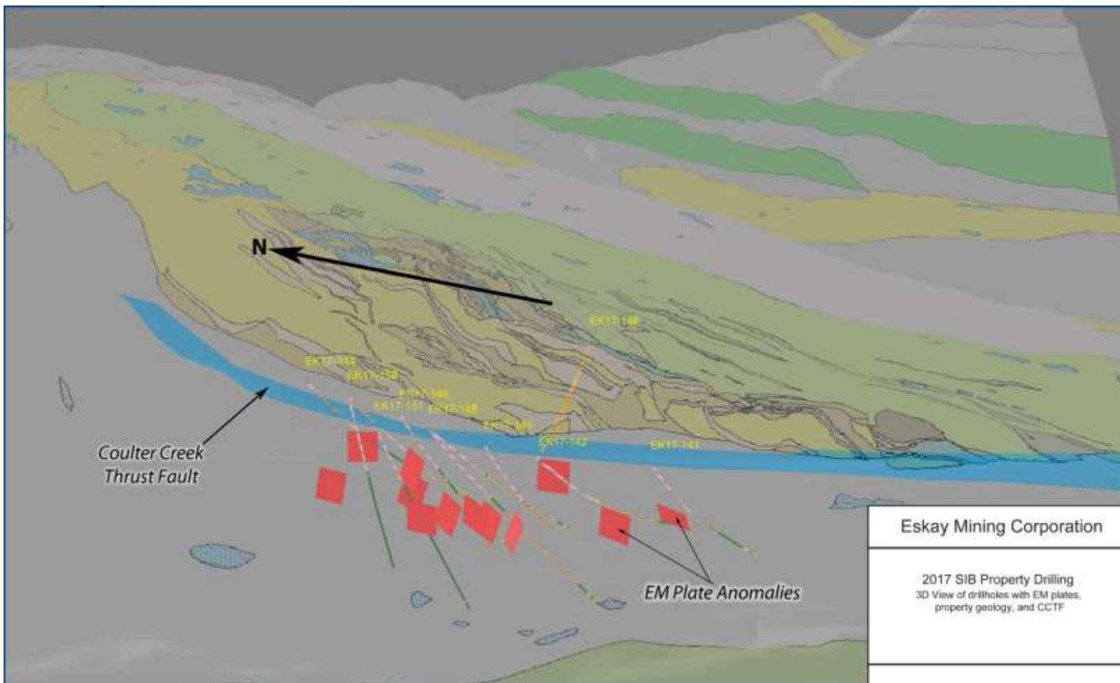
Figure 4: 3D perspective view of 2017 drillholes, showing CCTF and EM plate anomalies
